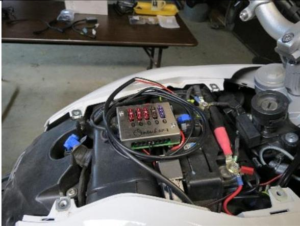
7) Its best to route cables is along each side and up under the plastic side covers, coming up next to the battery (see the heavy black cable, in picture).
