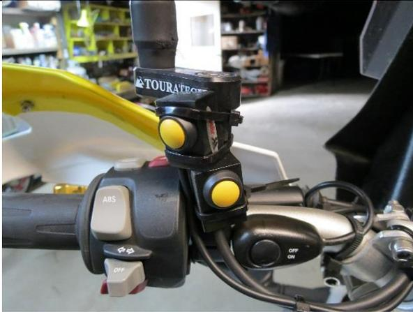
9) The Push to Talk Buttons are key features of the the Baehr systems. There are many ways to use them with communication devices, deciding ahead of the time is necessary to decide cable routing and what operates what.
