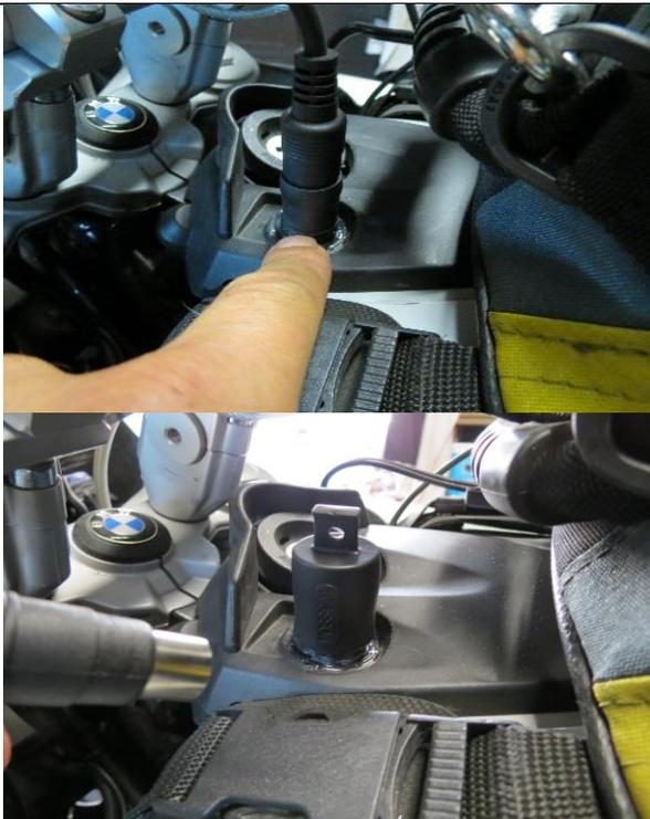
8) Remove the BMW power socket, and run the drivers helmet-cable up the left side of the bike and to the ignition-plate socket. A Dremel tool or small round-file is best, round the inside edge of the socket-hole, GO SLOW, and ensure the FEMALE end of the Verso-XL cable fits tightly into the modified socket hole. Secure the cable end with some soft but tough glue such as ShoeGoo, this will provide a watertight seal as well as strength.
